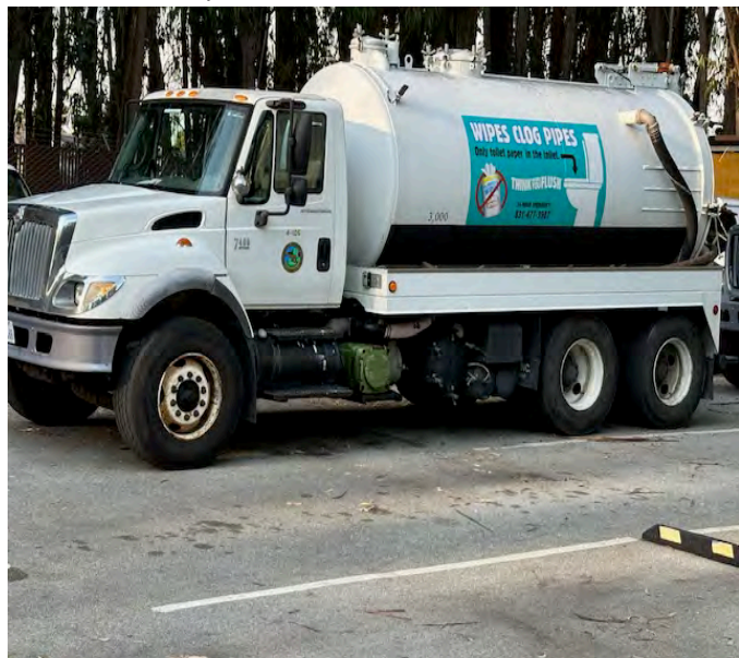
Photo 11: Corp Yard inspection (3,000-gallon combination truck – 3 in service and ready for deployment).
