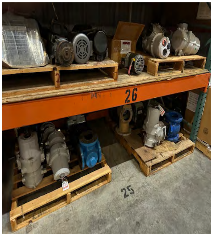
Photo 9: Corp Yard inspection (critical spare parts including check valves, isolation valves, and air release valves).
