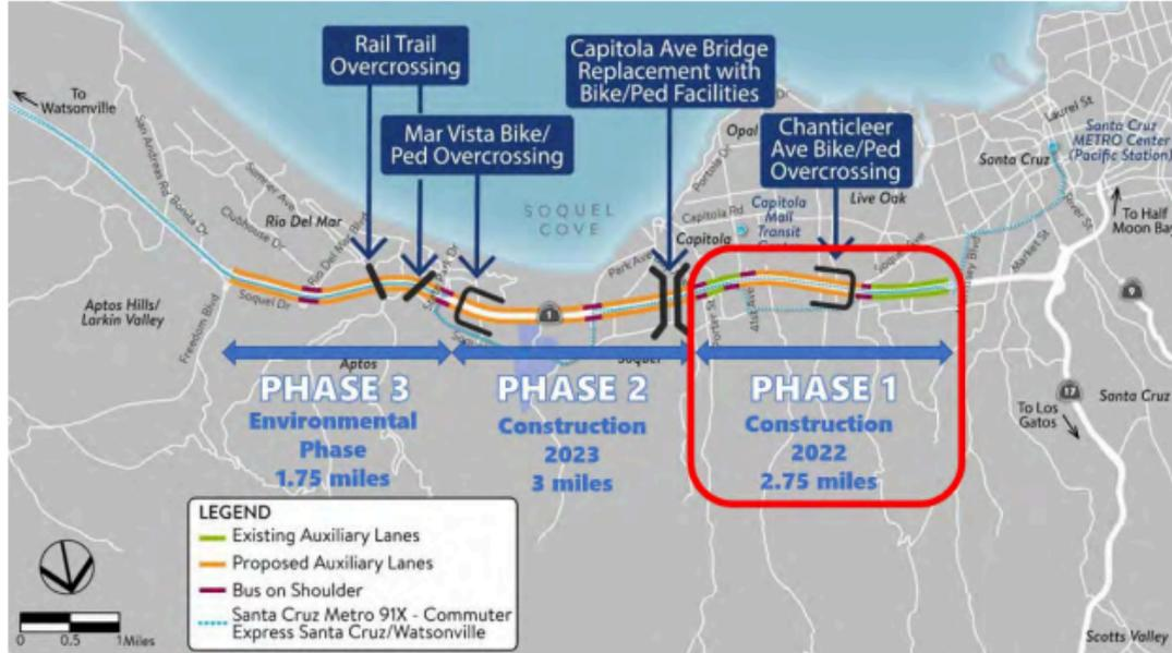
**Figure 1 - Phase 1 Project includes auxiliary lanes and a bus on shoulder facility in both directions of Highway 1 (41<sup>st</sup> Avenue to Soquel Drive), retaining walls, soundwalls, and a new bicycle/pedestrian overcrossing at Chanticleer Avenue**
