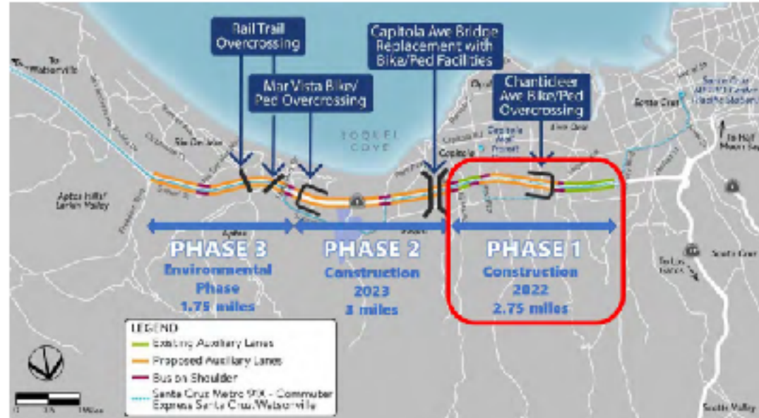
Figure 1 - Phase 1 Project includes auxiliary lanes and a bus on shoulder facility in both directions of Highway 1 (41st Avenue to Soquel Drive), retaining walls, soundwalks, and a new bicycle/pedestrian overcrossing at Chanticleer Avenue
